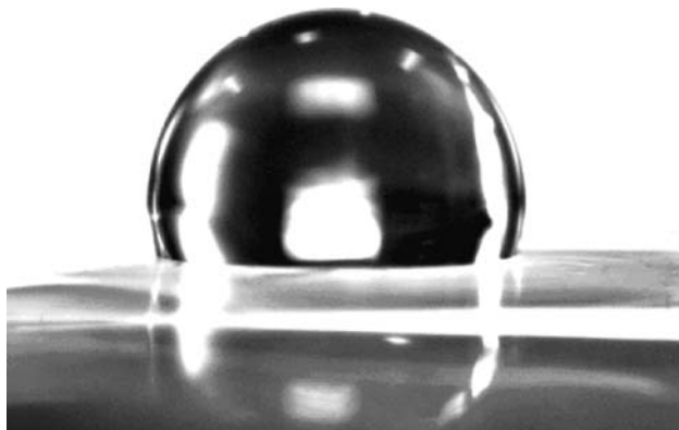
Fig. 2 A water droplet on a 1H, 1H-perfluorooctylamine-grafted nylon surface
